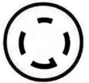
L14-30 250V GENERATOR
